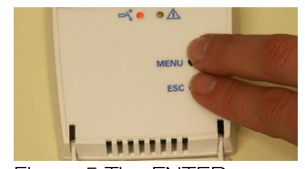
Figure 5 The ENTER command is done by pushing buttons MENU and ESC at the same time for about 14s.
