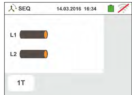
Fig. 25: Phase sequence check of 2T phases with terminal and remote lead
