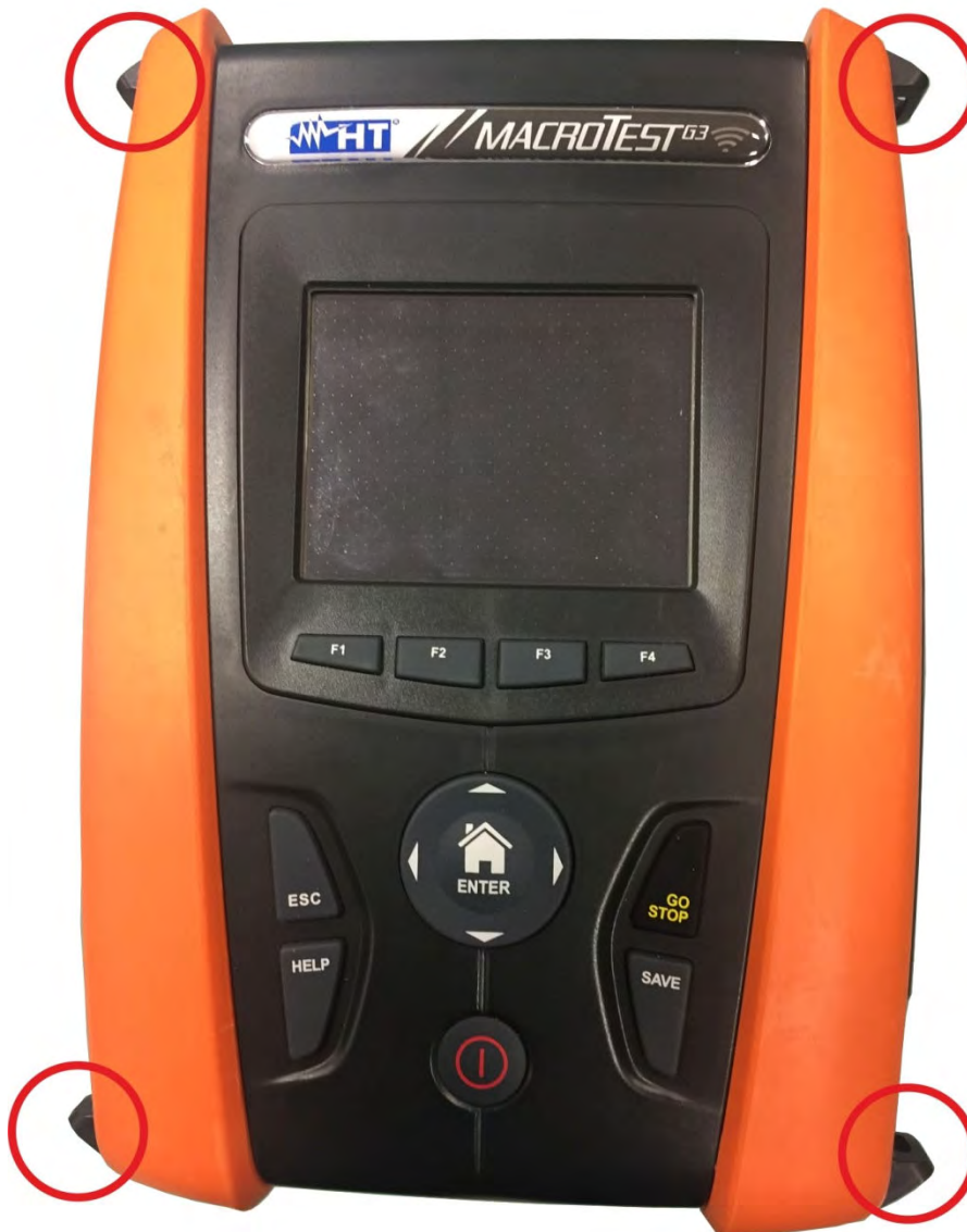
Fig. 42: Instrument with fitted half-shells and hooks
